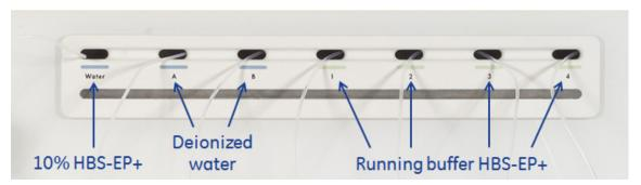
The only difference compared to the instructions in the software is that the tubing marked "Water" should be placed in the bottle with 10% HBS-EP+ solution:
