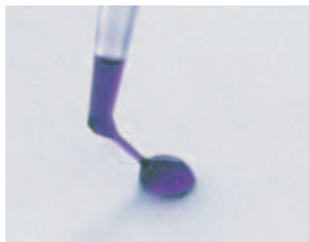
Fig 5. The viscous product of TempliPhi amplification can be difficult to pipette accurately. Dye was added to the TempliPhi-amplified product to increase DNA visibility in the photograph.
