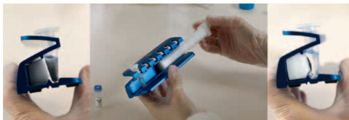
Fig 2. The high density of the beads allows rapid capture with MagRack 6.
