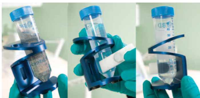
Fig. 3 MagRack Maxi showing the magnetic bar detached (left) and inserted (right).
