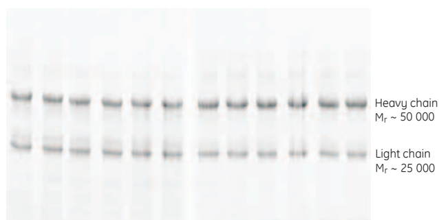
Fig 4. Purification of six samples in parallel with MagRack 6. The SDS gel (reducing conditions) was stained with Deep Purple™ Total Protein Stain and analyzed with ImageQuant™ TL software. The purity obtained for six replicate runs was above 90% (RSD < 2%).
