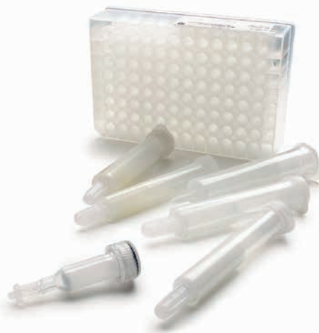
Fig 1. PD protein sample preparation products are prepacked with Sephadex G-25 Medium. The PD G-25 product range includes (from top to bottom), PD MultiTrap G-25, PD MiniTrap G-25 (two columns shown), PD MidiTrap G-25 (two columns shown), PD-10 Desalting Column, and PD SpinTrap G-25.
