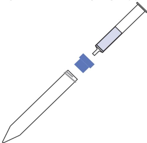
**Fig 1.** Assembly of column, adapter and collection tube.
