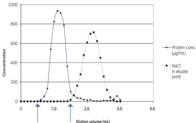
**Fig 2.** Removal of NaCl from albumin solution with PD MiniTrap G-25. The albumin is eluted in volume fractions between 0.5 to 1.5 mL (indicated by arrows).
