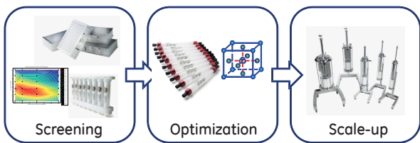
Fig 3. The recommended workflow is described in the figure. It starts with screening of conditions in high throughput formats, followed by optimization, preferably by applying Design of Experiments (DoE), in small columns and finally scale-up to large columns.
