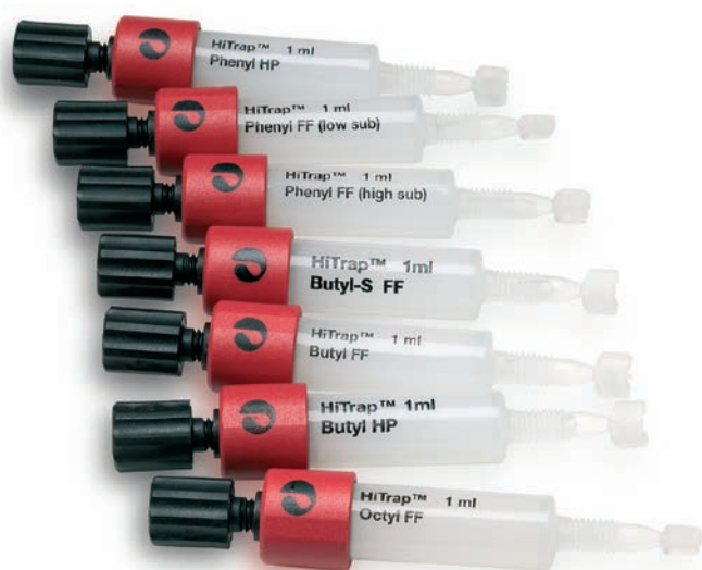
Fig 1. HiTrap HIC Selection Kit includes seven different HiTrap HIC 1 mL columns.
