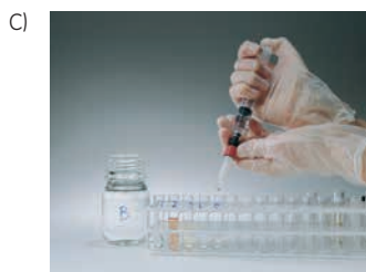
Fig 2. Using HiTrap rProtein A FF, HiTrap Protein A HP or HiTrap Protein G HP with a syringe. (A) Prepare buffers and sample. Re-move the column's top cap and snap off the end. Wash and equilibrate. (B) Load the sample and begin collecting fractions. (C) Elute and continue collecting fractions.
