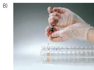
Fig 2. Using HiTrap rProtein A FF, HiTrap Protein A HP or HiTrap Protein G HP with a syringe. (A) Prepare buffers and sample. Re-move the column's top cap and snap off the end. Wash and equilibrate. (B) Load the sample and begin collecting fractions. (C) Elute and continue collecting fractions.
