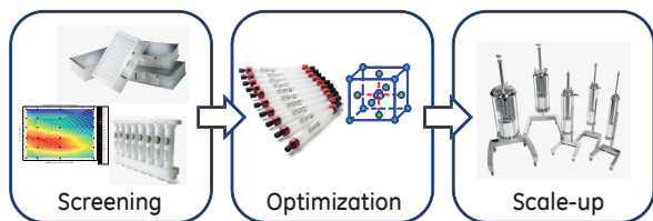
Fig 3. The recommended workflow is described in the figure. It starts with screening of conditions in high throughput formats, followed by optimization, preferably by applying Design of Experiments (DoE), in small columns and finally scale-up to large columns.
