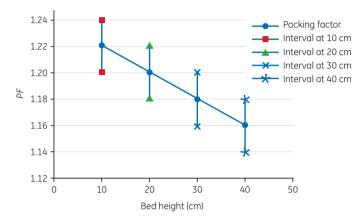
**Fig 2.** Bed height and packing factor curve for AxiChrom columns up to 600 mm, illustrating the packing factors' decreasing linearity for different bed heights. For each bed height, there is an acceptable interval for the packing factor. The packing factors are established for packing with 150 mM NaCl.
