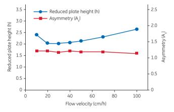
**Fig 8.** Reduced plate height and asymmetry values at different flow velocities for Capto S ImpAct packed to a bed height of 20 cm in a Chromaflow 600 column (CF = 1.10). These values should be regarded as examples. However, similar behavior can be expected for packed beds in other columns such as AxiChrom and BPG.
