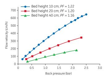
**Fig 5.** Pressure-flow curves for Capto S ImpAct in 150 mM NaCl packed in AxiChrom 300 to different bed heights using different packing factors. Capto S ImpAct can be run at 220 cm/h with a back pressure of less than 3 bar for bed heights up to 20 cm.
