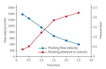
Fig 4. Column pressure and flow velocity during packing of a 20 cm bed height in Chromaflow 600 by the use of Chromaflow Packing Station Pack 100.
