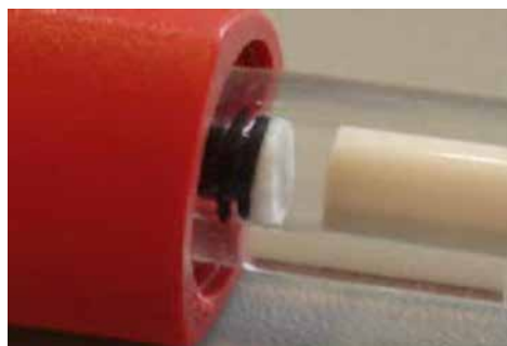
Fig 6. The maximum pressure over the packed bed is the maximum pressure the packed bed of chromatography medium can withstand without gap formation. This is not a fixed value.
