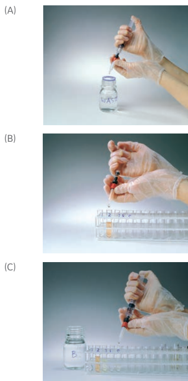
Fig 2. Using a HiTrap Q HP or HiTrap SP HP 1 mL column with a syringe. (A) Prepare buffers and sample. Remove stop plug from top of the column and snap off the end. Equilibrate. (B) Load the sample and begin collecting fractions. (C) Wash, elute and continue collecting fractions.
