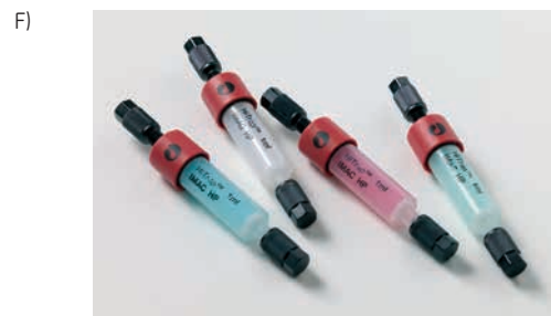
Fig 4 A-E. Purification of (histidine) 6 -tagged YNR064c expressed in Pichia pastoris on four different HiTrap IMAC HP 1 mL columns charged separately with metal ions A) Cu 2+ , B) Zn 2+ , C) Co 2+ , or D) Ni 2+ . Pools selected after SDS-PAGE of individual 1 mL fractions (not shown) are indicated. E) SDS-PAGE analysis: reducing conditions on ExcelGel SDS Gradient 8–18; Coomassie staining. F) HiTrap IMAC HP 1 mL columns charged with Cu 2+ , Zn 2+ , Co 2+ and Ni 2+ , respectively.
