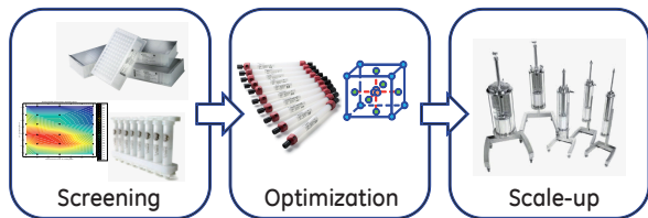
Fig 6. The workflow starts with screening of conditions in high throughput multiwell formats, followed by optimization, preferably by applying Design of Experiments (DoE), in small columns and finally scale-up to large columns.
