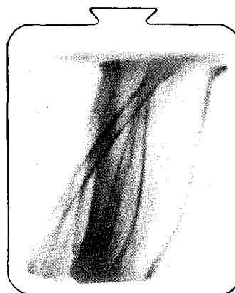
Example of a titration curve with PhastGel IEF 5–8. The gel was silver stained using the method described in development technique file number 210. The sample is beef muscle extract.
