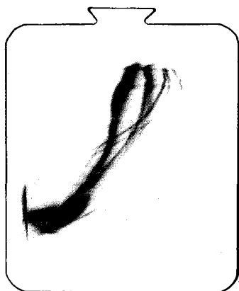
Example of a titration curve with PhastGel IEF 3–9. The gel was Coomassie stained using the method described in development technique file number 200. The sample is beef muscle extract.
