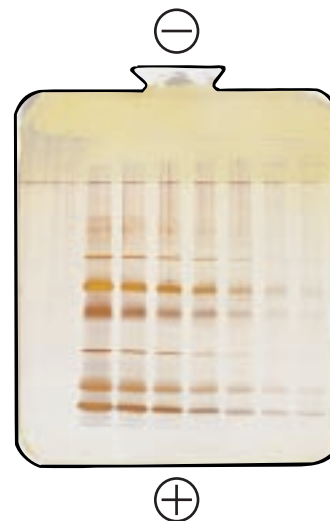
Fig. 2. Serial dilution of the LMW Calibration Kit (denatured) on PhastGel gradient 10–15 with SDS buffer strips. Each vial contains approximately 100 µg of each of the proteins listed below. The dilution volume/vial is, starting from the left: 1.6 ml, 3.2 ml, 6.4 ml, 12.8 ml, 25.6 ml, 52 ml and 102 ml. The samples were applied in 1 µl volumes to each of 7 lanes (the first lane is empty).
