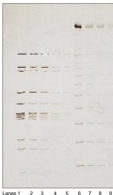
Fig. 4. DNA markers run on GeneGel Excel 12.5/24 and stained with DNA Silver Staining Kit. Lanes 1–5, \Phi X-174-RF DNA Hinc II; lanes 6–9, 100 Base-Pair Ladder. The sensitivity limit was 100 pg for the 495 bp fragment band.
